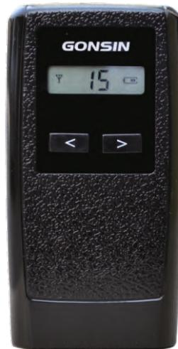
TC-RF J04S/08S/12S/16S wireless simultaneous receiver serves to receive audio signal. Participant use the receiver to select a required audio channel and wear a headphone to hear interpretation. Volume is adjustable. Signal strength, battery capacity, selected channel, etc can be displayed on the LCD screen.
